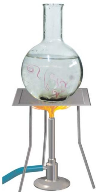
**Fig. 4.9** Convection of heat in water
