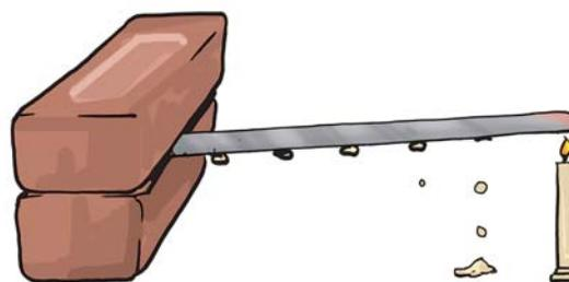
**Fig. 4.7** Flow of heat through a metal strip
